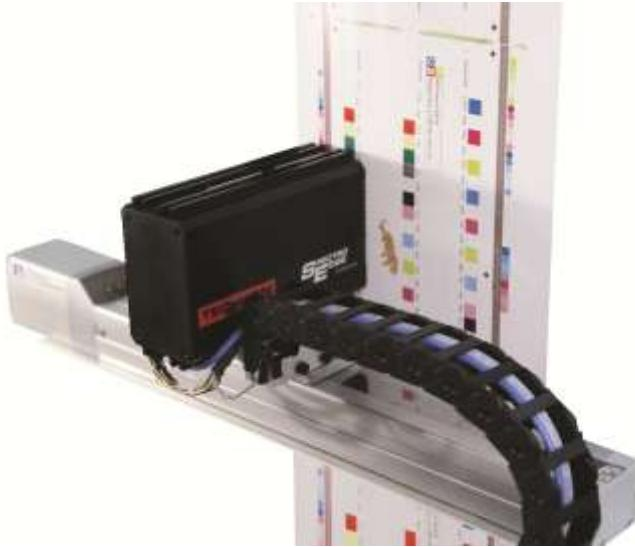
Typically this would require a color bar printed on the media along the direction of the press run, likely on either side of the web such that the results of the plate pressure can be monitored. The bar consists of solid and tint patches of each process color as well as overprints and gray balances. There may also be one or several (possibly all) spot colors included in the color bar to ensure that special colors such as those used for company logos are reproduced accurately.
